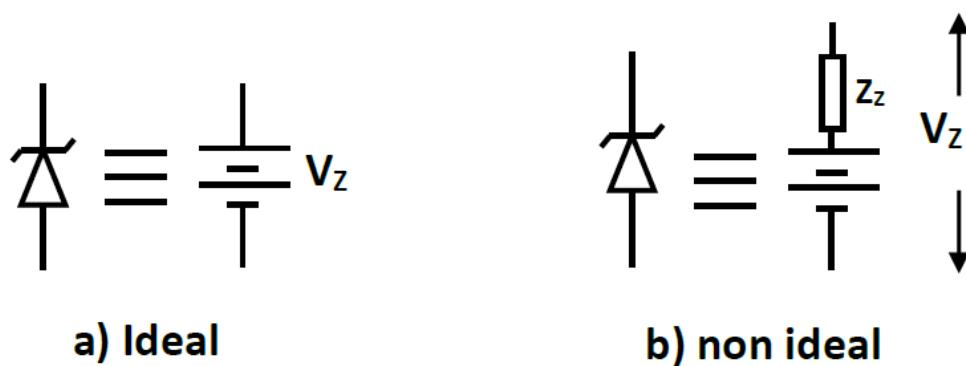
It has a constant voltage drop equal to nominal zener voltage. This constant voltage drop is represented by a dc voltage source even though the zener diode does not actually produce an emf voltage. The dc source simply indicates that the effect of reverse breakdown is a constant voltage across the zener terminal.
