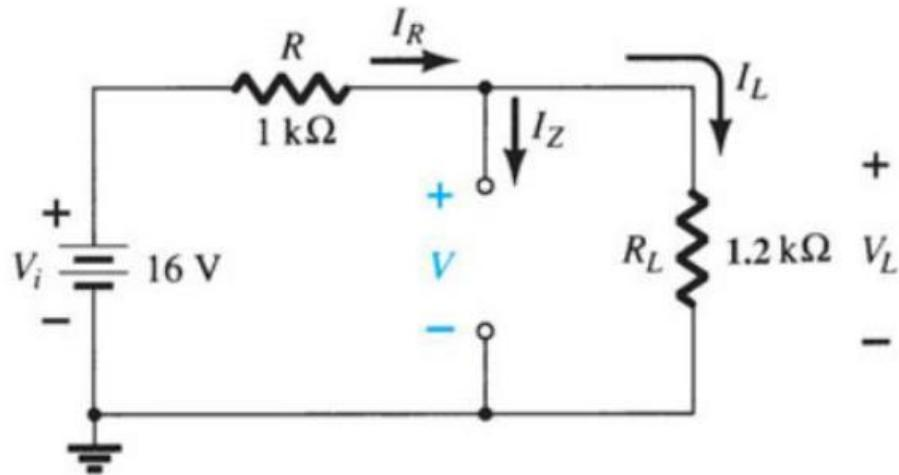
$$V = V_L = V_i \times \frac{R_L}{R + R_L} = 16V \times \frac{1.2k\Omega}{1k\Omega + 1.2k\Omega} = 8.7272 \text{ V}$$
