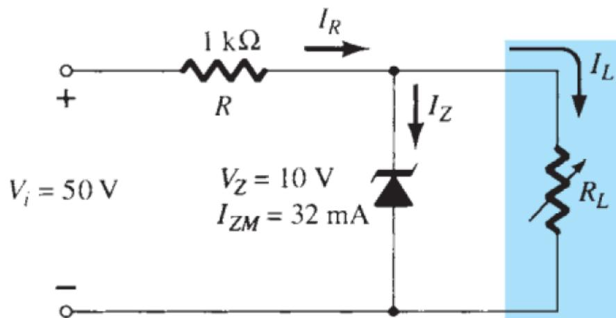
Solution: To determine the value of  $R_L$  that will turn the zener diode ON
