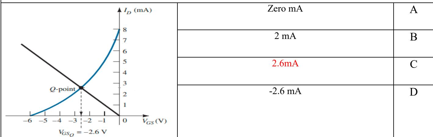
**Q45.** For the transfer characteristics of JFET (voltage divider circuit) shown the value of  $I_{DQ}$ ?
