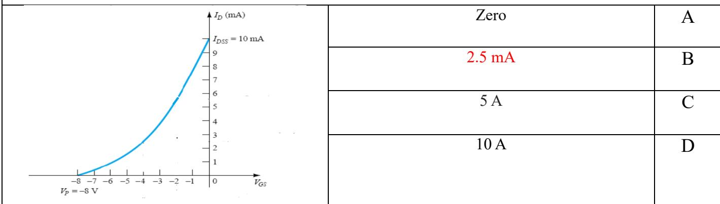
**Q19.** What is the value of drain current when  $V_{GS} = \text{pinch-off voltage } V_p$ ?
