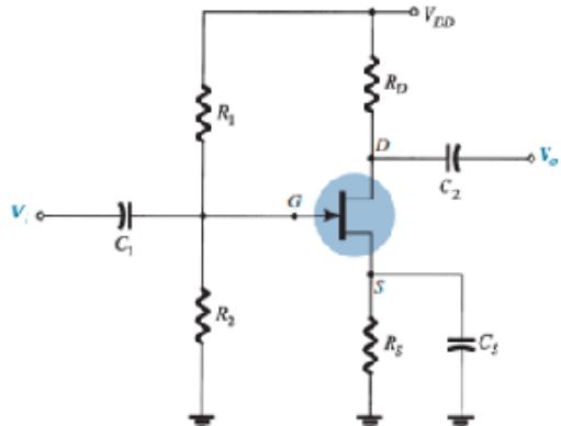
$$V_G = \frac{V_{DD} R_1}{R_1 + R_2}$$
