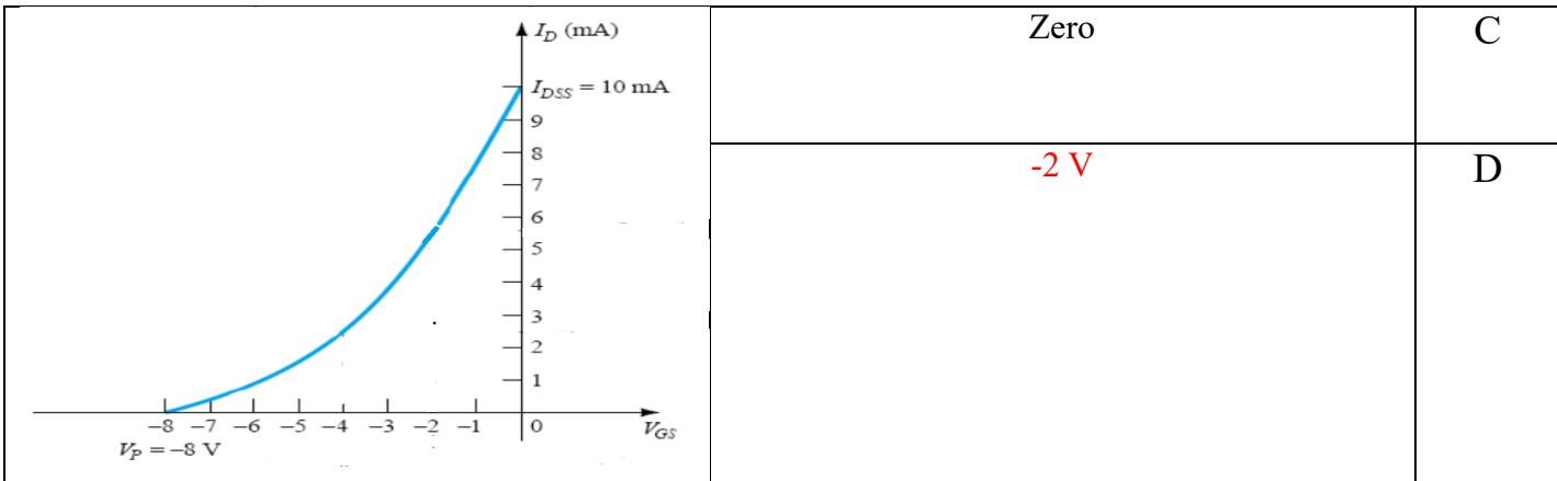
**Q17.** For the FET transfer characteristics, when  $I_D = I_{DSS}/2$ , then  $V_{GS}$  is .....
