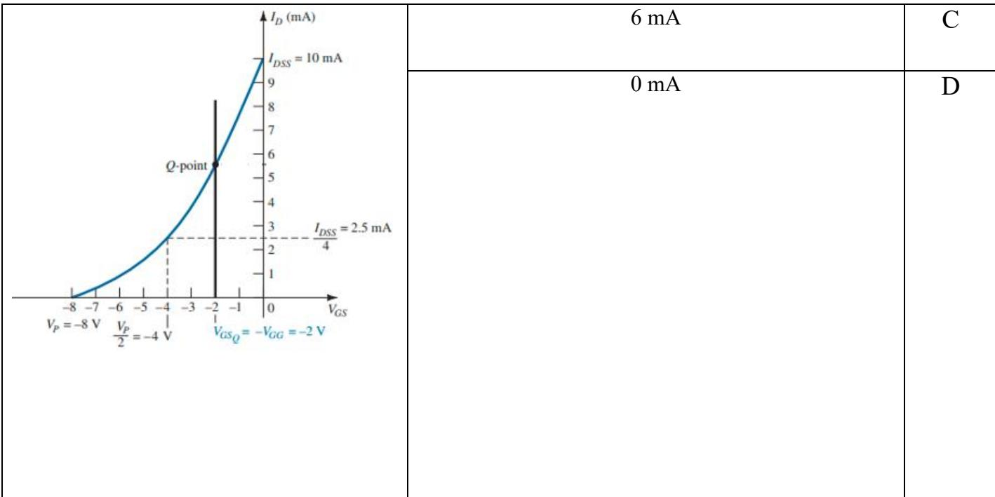
**Q44.** For the transfer characteristics of JFET (self bias circuit) shown the value of  $I_{DQ}$ ?
