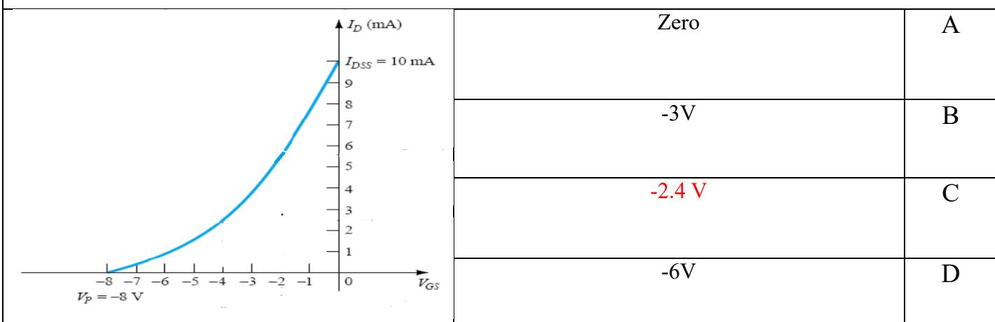
**Q18.** For the FET transfer characteristics, when  $V_{GS} = V_p/2$ , then  $I_D =$  .....
